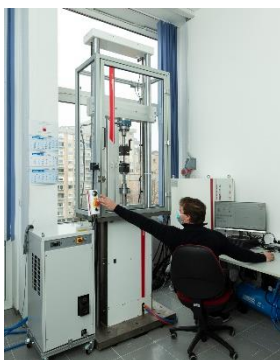
Figure 2: Multiaxial static and dynamic test rig (Photo: IFP, d.o.o.)
