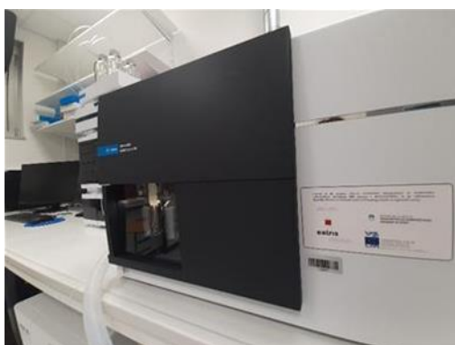
Picture 1: Liquid chromatograph coupled with a high-resolution mass detector at the time of flight
