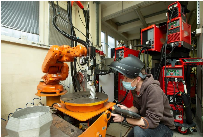
Figure 7: Advanced robotic 3D metal printer and robotic winding system (Photo: IFP, d.o.o.)
