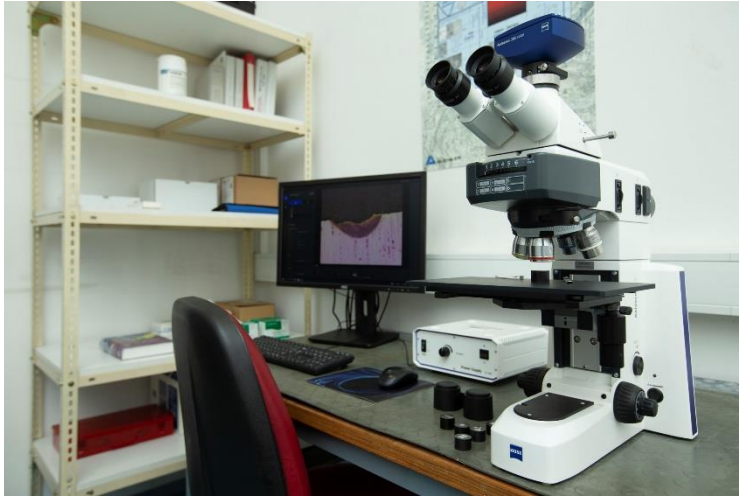
Figure 5: ZEISS Axioscope 5 metallurgical optical microscope with accessories (Photo: IFP, d.o.o.)
