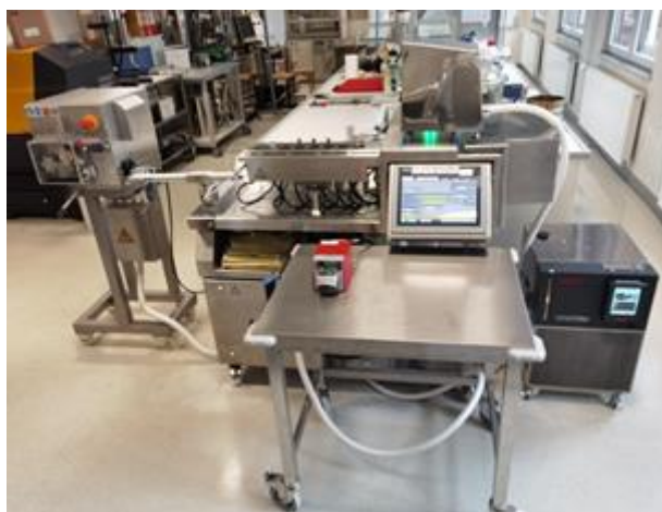
Picture 6: Leistritz ZSE 12 HP-PH twin screw hot melt extruder for hot melt extrusion (HME) and twinscrew granulation (TSG)
